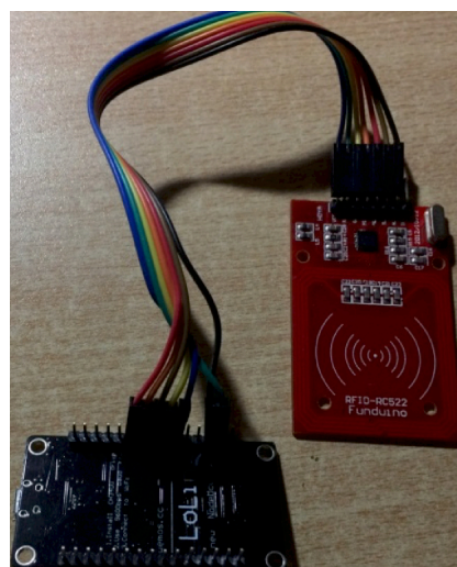
Figure 6. The physical realization of WiRF reader.
